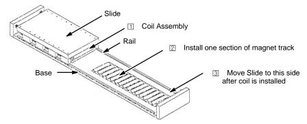
3. Hold the slide with a firm grip and move it over the magnet track section/shim.
